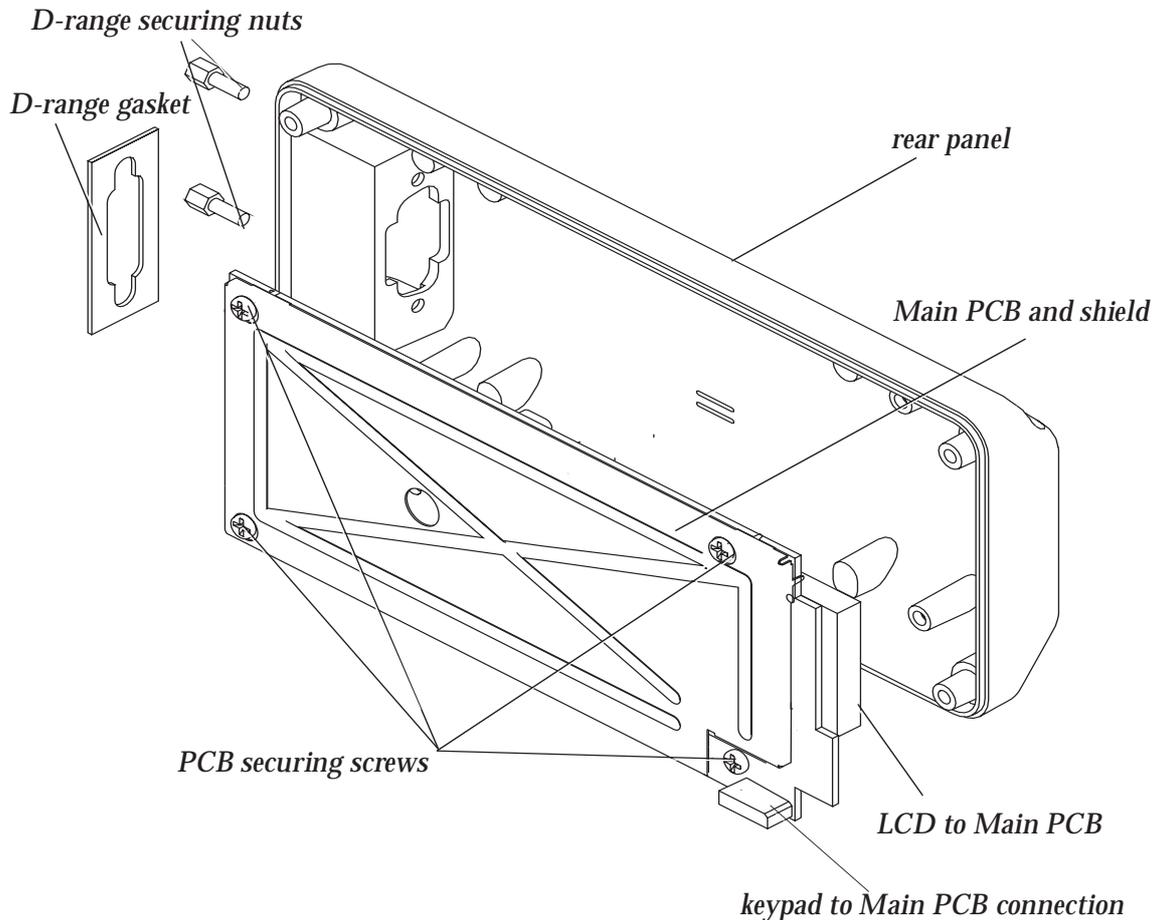
**Figure 4.8** *Fitting the Main PCB and Shield to the Rear Panel - Internal View*
