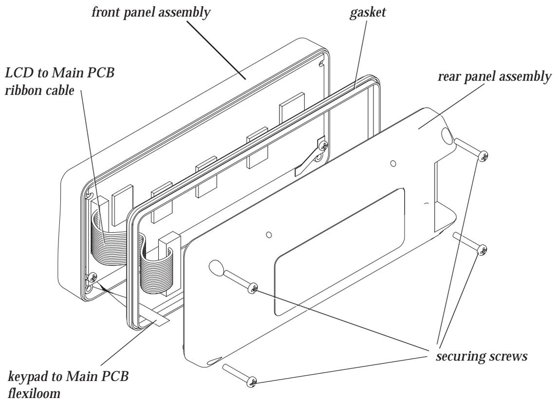
**Figure 4.3 Disassembling the MDT - Rear View**
