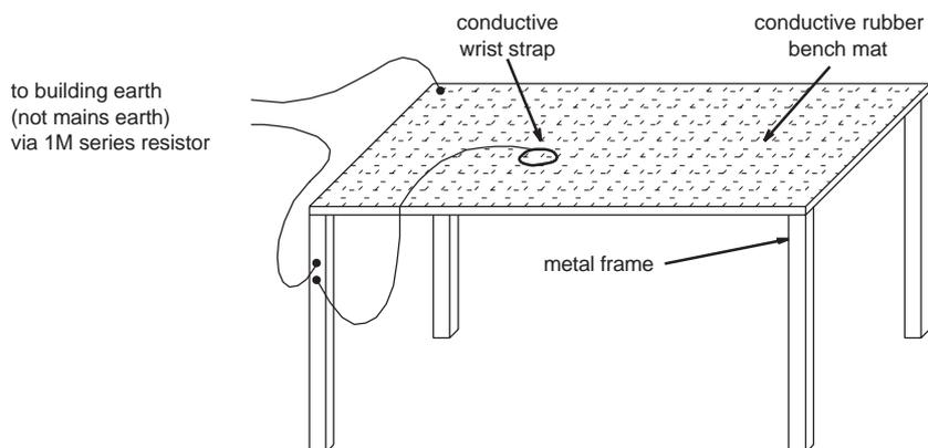
**Figure 4.1** Typical Antistatic Bench Setup
