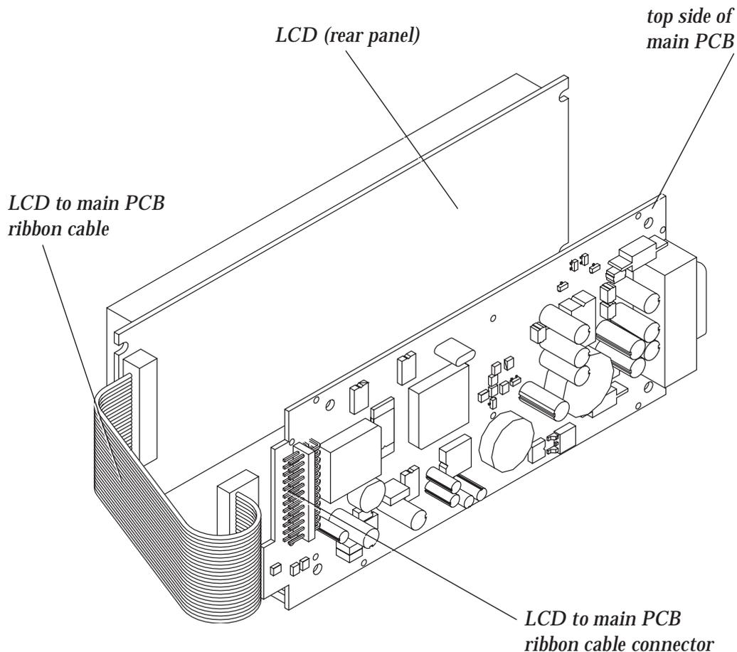
**Figure 4.9** Connecting the LCD to Main PCB Ribbon Cable
