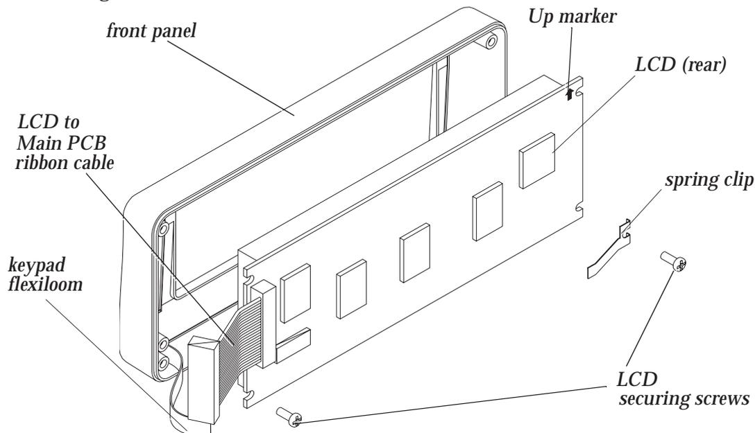
**Figure 4.7 Fitting the LCD to the Front Panel - Internal View of Front Assembly**
