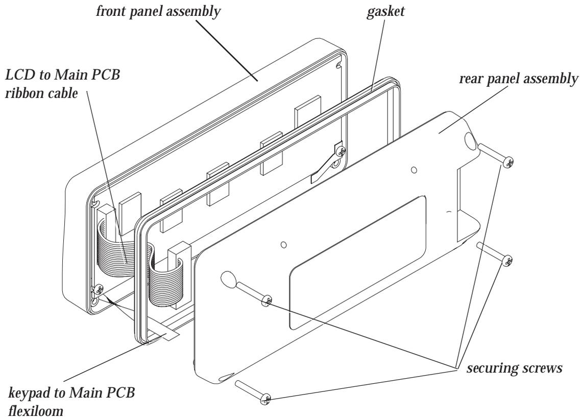
**Figure 4.10 Assembling the MDT - Rear View**
