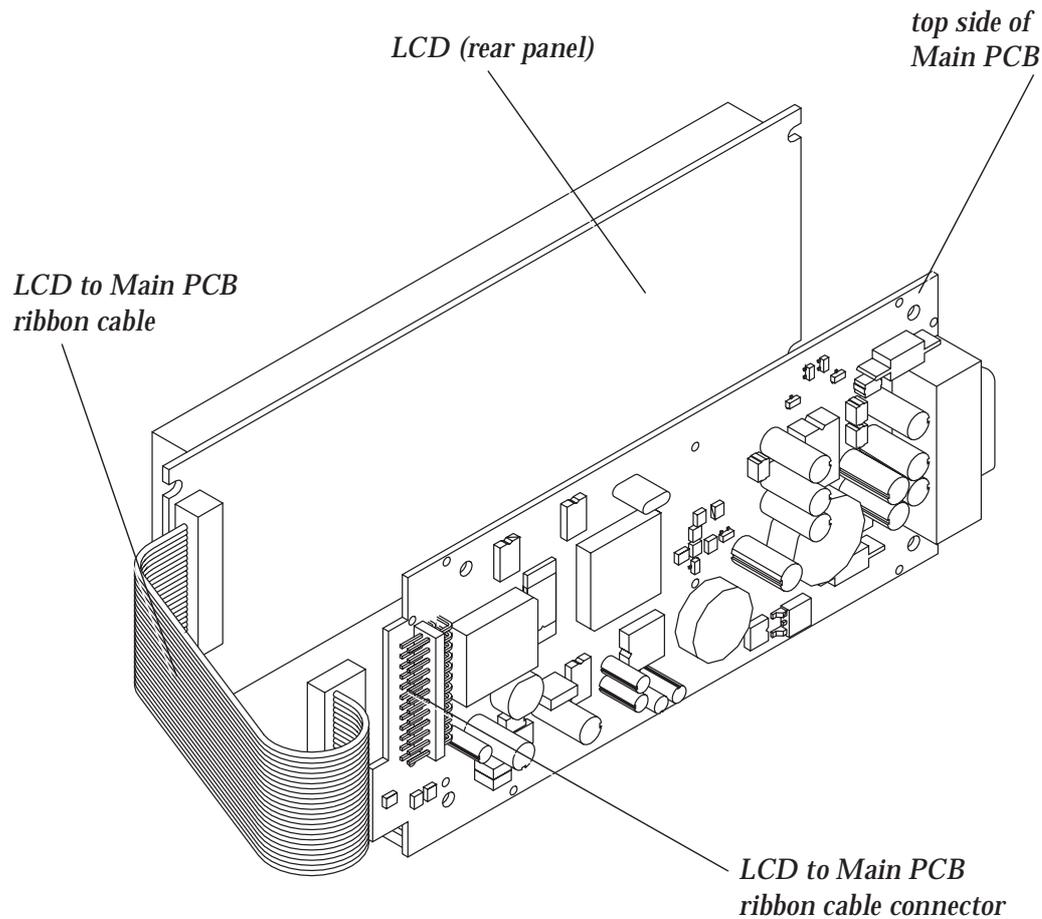
**Figure 4.5** *Disconnecting the LCD to Main PCB Ribbon Cable*
